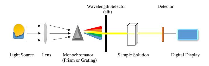
Figure 2. Basic components of a spectrophotometer  $\tilde{a}$
